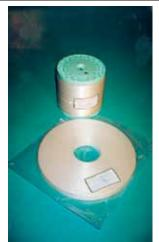
The storage room must be frozen, ventilated, and must protect the tape from the light.
